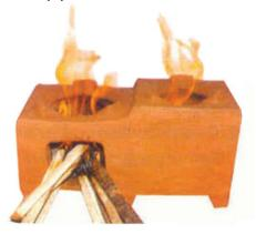
The TNAU double pot portable chulha (chimneyless) is made with two walls Around the first pot, an annular chamber having a width of 2.5 cm is left and the outer wall is constructed. The outer wall is also extended to cover the second pot in which case the annular chamber width is 3.5 cm, because of the smaller diameter of the second pot hole. Two secondary air inlets are made, one on the outer wall with rectangular shape (17 cm x 1 cm) near the combustion chamber and the other at the
